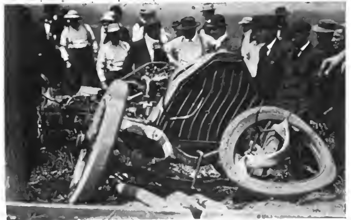
WRECK OF LYTLE CAR CAUSED BY BURSTING TIRE.
